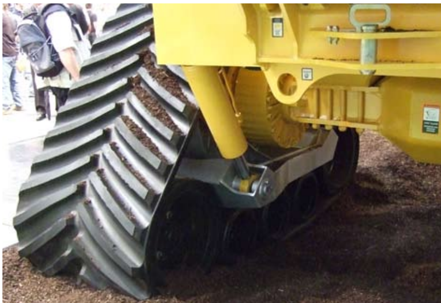
ill. 3.11.3: Tracks with a limited rotation, controlled by a hydraulic cylinder.
