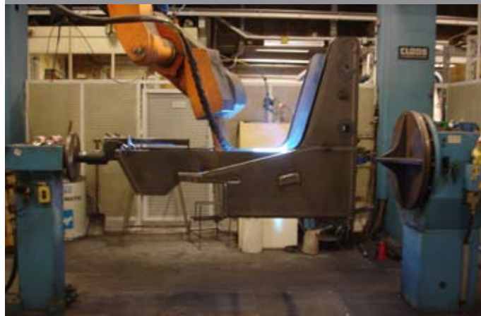
ill. 1.1.2: A welding robot controlling the process by itself.
