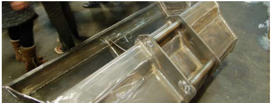
ill. 3.10.2. Shovel made of welded metal sheets.
