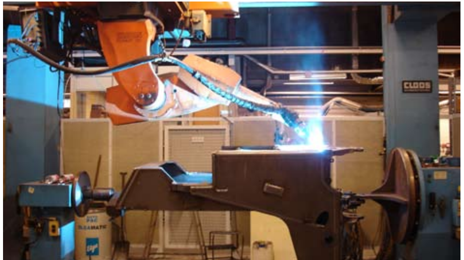
ill. 3.10.1. The welding machine at Hydrema, Støvring.
