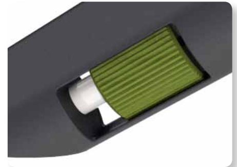
ill. 3.38. Numerous small grooves indicate precision and slow movement.
