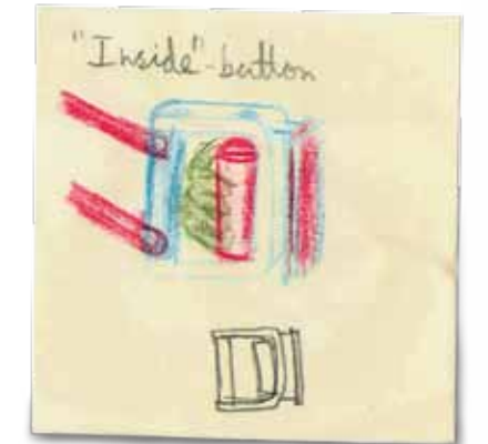
ill. 3.44. An earlier more complicated button that required activation in a less intuitive and more difficult approach.
